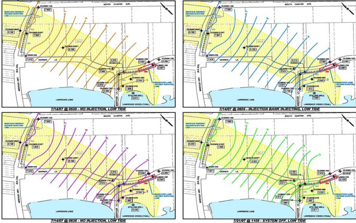
**Figure 4 Groundwater Elevation Contours (IB6)**
