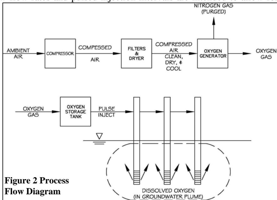
Each injection well is connected to the oxygen injection system with high density polyethylene tubing. An oxygen injection cycle begins by displacing water from the injection well followed by oxygen flow through the slotted PVC and filter pack. The filter pack acts as a diffuser by creating small bubbles of oxygen gas which disperse into the surrounding formation due to a pressure differential. A schematic showing the general process flow is shown in Figure 2.
